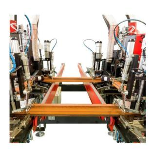
All the necessary operations are therefore carried out automatically, **milling** with the High Speed System, **positioning** at the operating levels, **cyclical casting**, **compression** and **cooling** and, at the end of the process, release with finished profiles.
